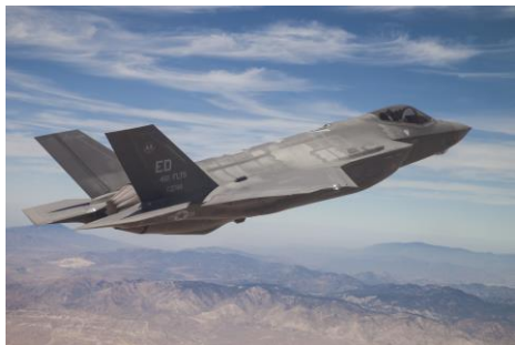
The F-35A is optimized to be a multi-role fighter, with the ability to perform air-to-air; air-to-ground; and intelligence, surveillance and reconnaissance (ISR) missions.
